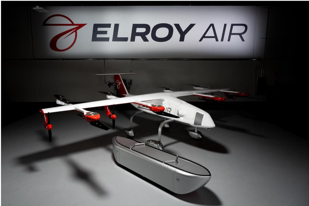
In January 2022, Elroy Air unveiled the design of their pre-production Chaparral C1 vehicle, an autonomous VTOL aerial cargo platform. It has a 300 lb capacity and a 300 mile range.
