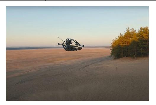
The futuristic machine, which resembles a one-person flying chair and is made from aluminum and carbon fiber is powered by eight electric motors and can reach a top speed of 63 mph or 102 km/h with a maximum flight time of 20 minutes. Make sure you land in time before a crash landing on land or a splash landing on water!
